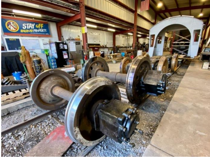
No. 576's new pilot wheels and repaired trailing truck wheels back in the steam shop. Submitted by Joey Bryan
