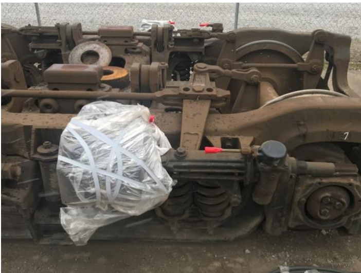
A trucks or west end of 1266 rolled out for inspection and repairs (above and upper right)
