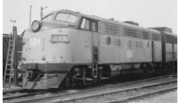
Photo above shows Bessemer & Lake Erie F7A 719A that TCRM has just purchased. It was in daily operation in Conneaut OH as recently as mid-December 2000. Arrangements are being made to move the locomotive to Nashville. EMD builder's number of the unit is 16591, built in 1952. Quite a coincidence that Gene Turnage's F7B is B&LE #719-B, eh? Photo E-mailed by Steve Tomblin, unit information from Steve Johnson
