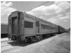
Above is a view of the ex Broadway Dinner Train power car 514. The car is spotted on our new maintenance spur track. We plan to have 2 large generator sets in this car along with a larger diesel fuel tank and state-of-theart electronic controls, making it our Super Power Car. Digital Photo by **Terry Bebout** on 24 June 2000.
